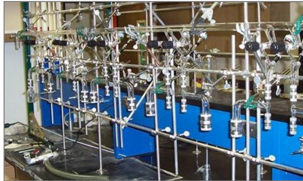
Cryogenic vacuum distillation 30-90 minutes per sample
