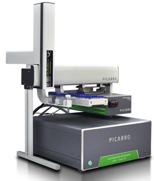
CRDS Direct measurement of Water 10-40 minutes per sample
